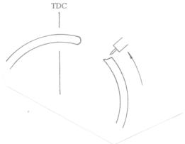
Secondly, the standard technique of feathering the end of the bead to be tied-in should be reduced to a maximum of 3mm. This minimises the length of weld produced without underbead flux protection (since the keyhole, by which flux flows to reach the bead underside, closes up). An alternative technique involves no feathering but utilises a current surge to ensure satisfactory tie-in with minimal potential loss of underside flux protection.
