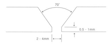
Typical preparations are illustrated above, it is important to maintain sufficient root gap to ensure adequate underbead slag protection. As with solid wire TIG welding, filler addition has to be balanced:
