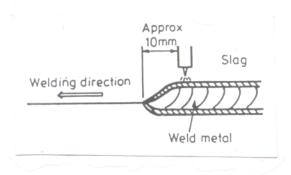
If cold, the top slag should be removed, but not the underside, for a distance of about 10mm. Inclined vertical-up welding tends to give easier keyhole reformation in difficult or narrow gap stop/start positions.
