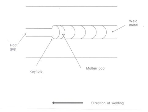
In principal, Metrode SUPEROOT 316L works like a covered electrode inside out. However, as with all TIG welding there is independent control of heat source (arc) and filler, allowing the welder to work with variations in fit up, root gap and welding position.
