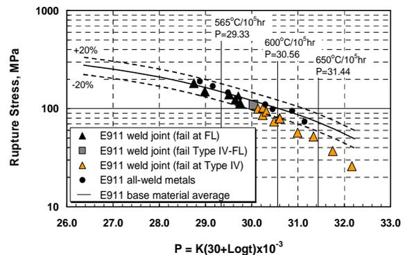
Figure 7. E911 transverse joint tests in comparison with all-weld metal and base material (C=30)
