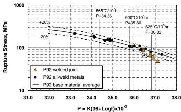
Figure 6 – P92 transverse joint tests in comparison with all-weld metal and base material (C=36 )
