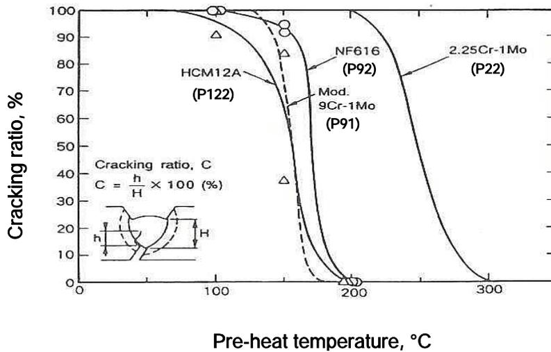
Figure 4. Y-groove test result of P92 weld metal and comparison with other Cr-Mo steels, including P91, P22 and P122 [11]
