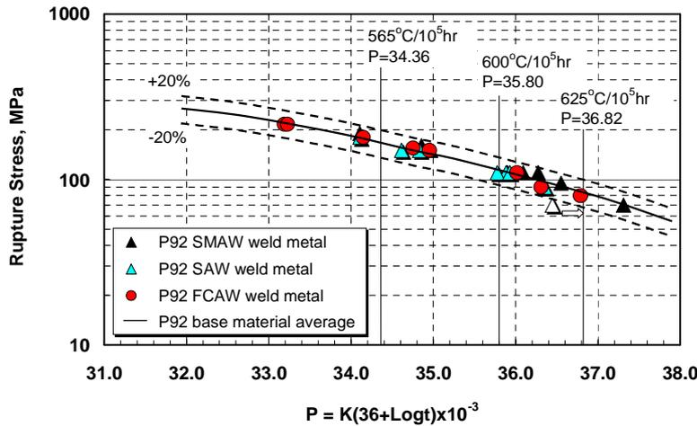
Figure 5. Larson-Miller plot of P92 base metal and weld metals with C=36
