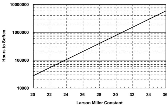
Figure 8. Estimated duration of alloy strength start softening vs Larson-Miller constant [13,14] (Operating temperature: 615°C; Tempering temperature: 760°C )
