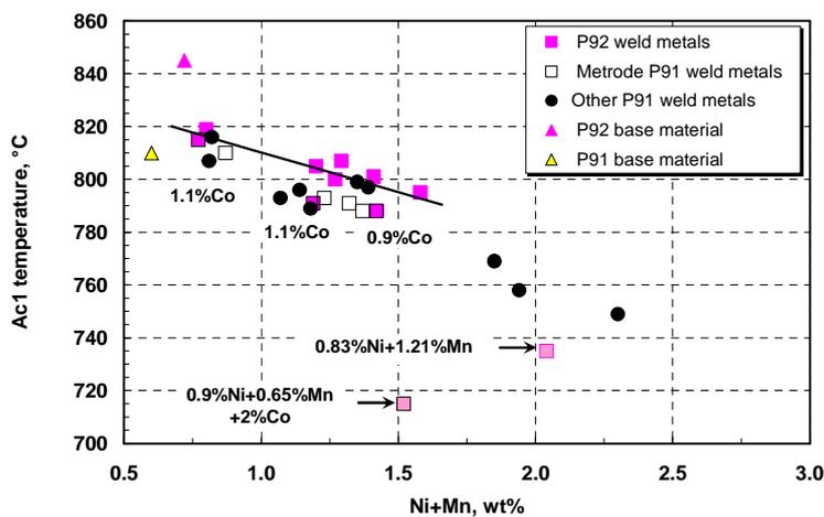
Figure 2. Effect of Ni and Mn on Ac1 temperature of P92 weld metals
