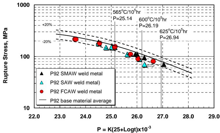
Figure 10. Larson-Miller plot of P92 base metal and weld metals with C=25
