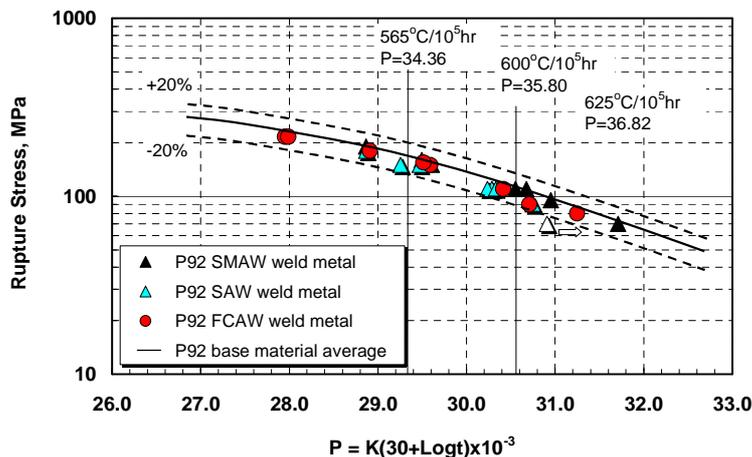
Figure 9. Larson-Miller plot of P92 base metal and weld metals with  $C=30$
