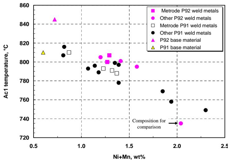
Figure 1. Ac1 temperatures of P92 and P91 weld metals and the effect of Ni+Mn content
