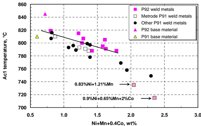
Figure 3. Effect of Ni, Mn and Co on Ac1 temperature of P92 weld metals
